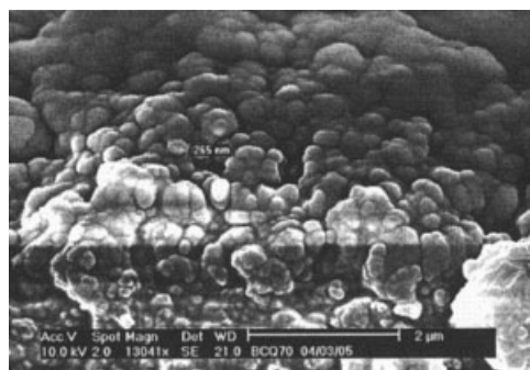
Figure 3 SEM picture of the complex support surface.
